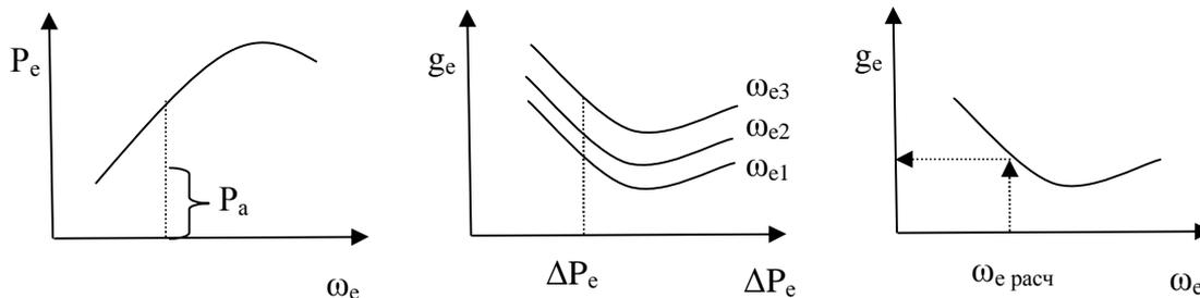
$$\omega_e = \frac{V_a \cdot i_{kn} \cdot i_0}{r_k}, [\text{рад/с}]; \quad \Delta P_e = \frac{P_a}{P_e} \cdot 100, \quad \%$$
